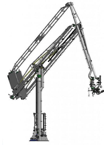
Figure 11. CO 2 loading and unloading arm
